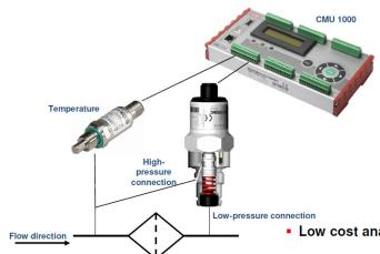
Condition monitoring of filter pressure drop
